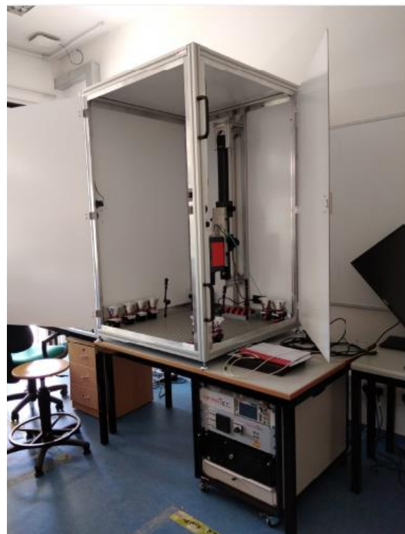
Manufacturer: INFRA TEC Model: PV-LIT Inspection system DLIT + ILIT (with ImageIR 8325 camera)
