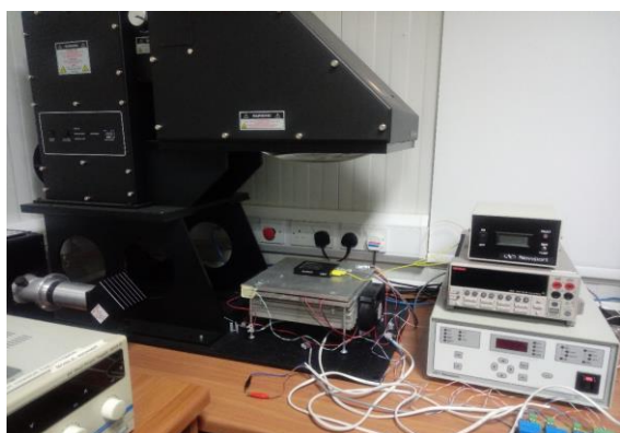
Manufacturer: Oriel, Newport Model: Sol3A Class AAA Solar Simulator
