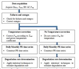
Figure 3: Degradation rate determination algorithm procedural flow chart.
