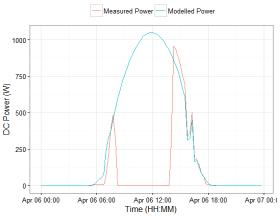
**Figure 9:** Measured and modelled power of a PV system during the FDR testing phase.
